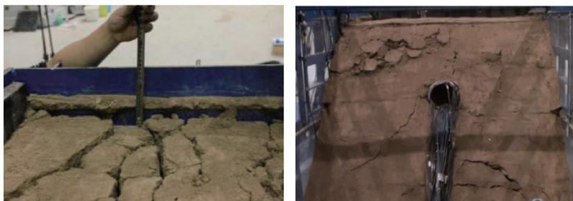
**Figure 4** Development stage of local earthquake damage
